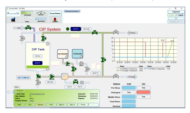
The system provides CIP for target (plant/production) system. There is full automatic operation, including the ability to change to any step in the Program at any time. The program will run according to selections and using the setpoints chosen and will automatically stop on critical alarms and resume on Alarms reset and resume commands..
